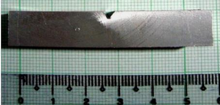
A rectangular metal specimen with a notch, placed on a green grid with a ruler below it. The ruler shows a length of approximately 5.5 cm. |
