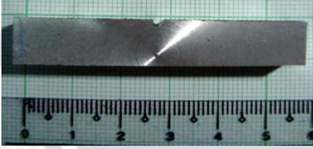
A rectangular metal specimen with a notch, placed on a green grid with a ruler below it. The ruler shows a length of approximately 5.5 cm. |
