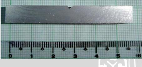
A rectangular metal specimen with a notch, placed on a green grid with a ruler below it. The ruler shows a length of approximately 5.5 cm. |
