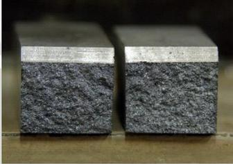
Two pieces of the specimen after impact, showing a clean fracture surface.   |
