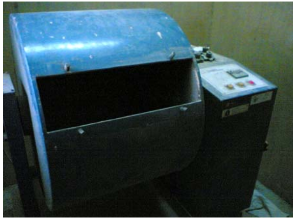
Gambar 7. Uji Keausan Los Angeles
