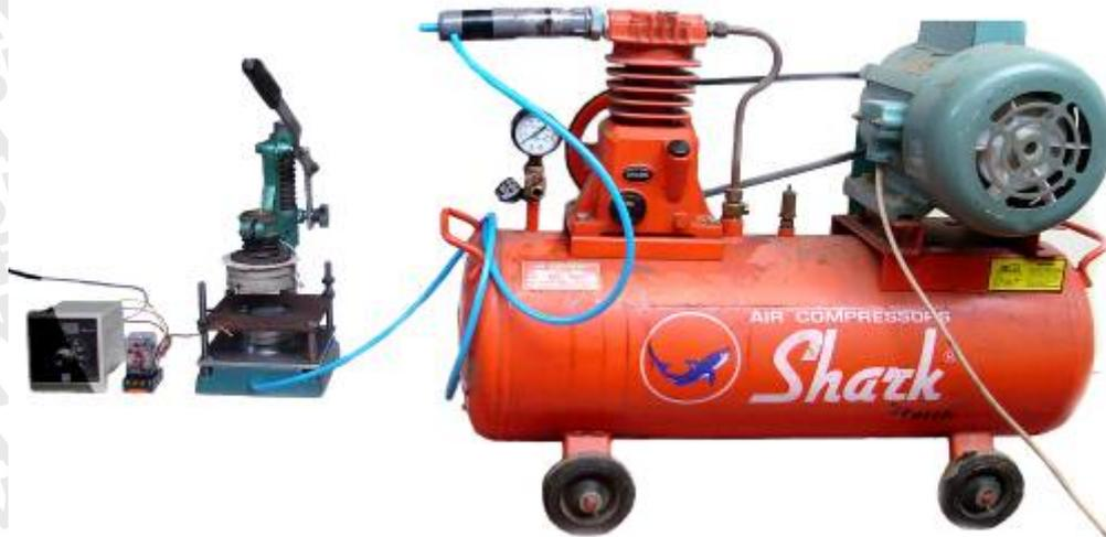
Gambar 3.1. Instalasi mesin *vacuum forming*
