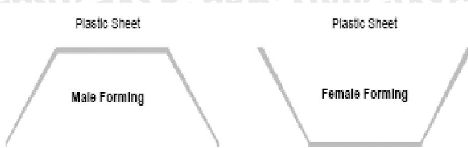
Gambar 2.8. Distribusi ketebalan antara *male mold* dan *female mold*
