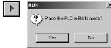
Figure 2-12 Placing the S7-200 in RUN Mode
