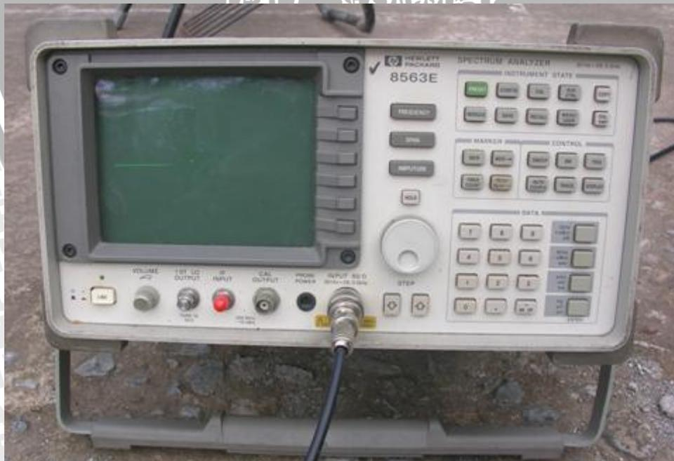
Spectrum Analyzer 8563E 30 Hz - 26.5 GHz Hewlett Packard
