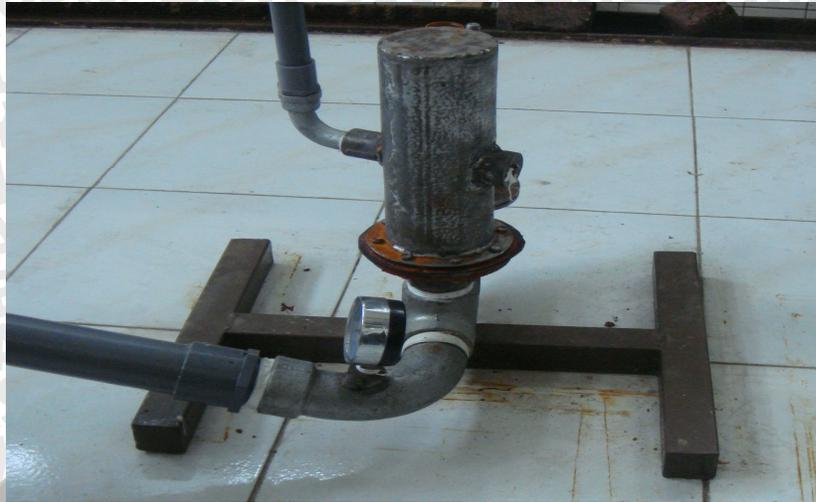
Gambar 3.1 Pompa Hydraulic Ram
