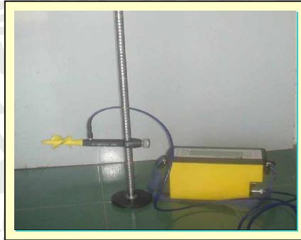
**Gambar 2.1 Current Meter Digital**
