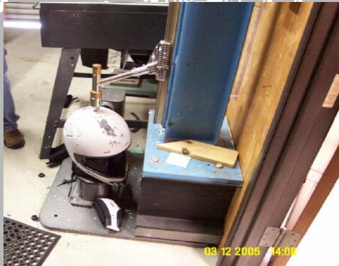
Gambar 2.7 Uji helm metode Penetration Test .
