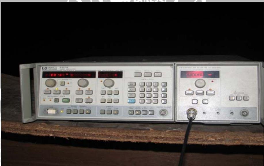
Gambar 20. Hewlett Packard RF Sweep Oscillator 8350B 0.01KHz– 26.5GHz
