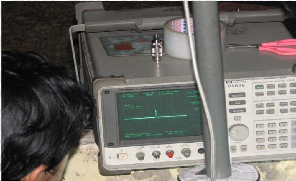
Gambar 21. Hewlett Packard Spectrum Analyzer 8563E 30Hz – 26.5GHz
