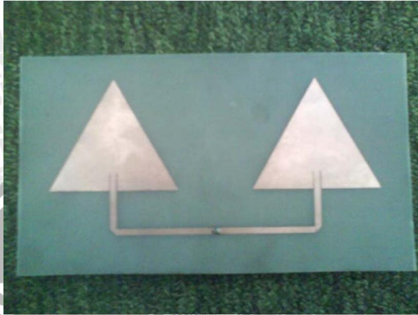
Gambar 17. Antena Mikrostrip *Equilateral Triangular Array* Dua Elemen
