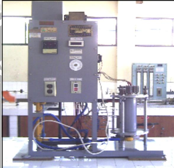
Gambar. 3.2. *Thermal Conductivity Measuring Apparatus*
