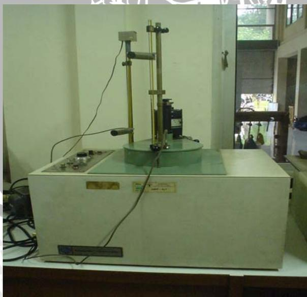
Gambar 3.5 Bomb calorimeter
