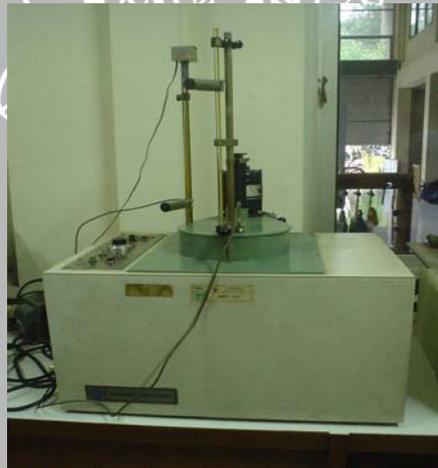
**Gambar 14. Instalasi Bom Kalorimeter
