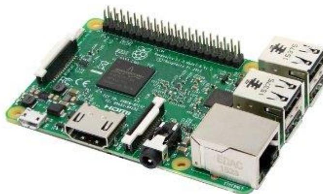
**Gambar 2. 12 Raspberry Pi 3 Model B**
