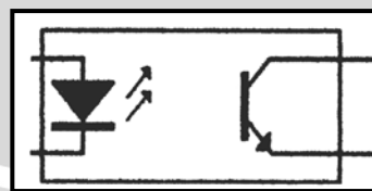
Gambar 2.19 Diagram rangkaian optocoupler Sumber : Motorola Semiconductor Technical Data 7:2
