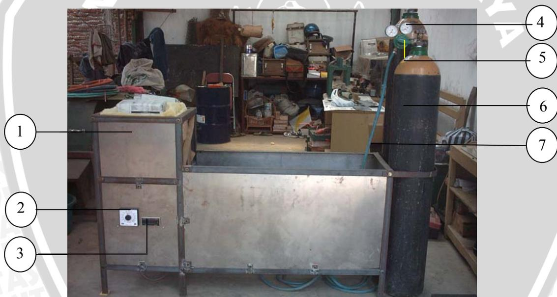
Gambar 3.1. *Fluidized bed furnace*
