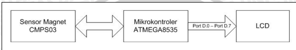
Gambar 5.1 Diagram Blok Pengujian Sensor Magnet CPMS03
