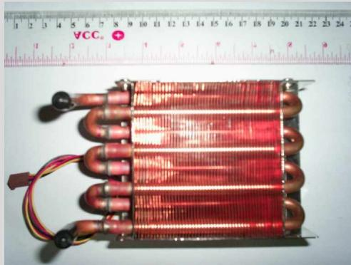
Gambar 2.4 Radiator sistem pendingin *processor*
