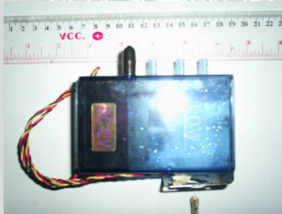
Gambar 2.6 Water pump sistem pendingin processor
