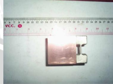
Gambar 2.5 Waterblock sistem pendingin processor
