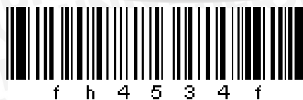
Gambar 2.16 Barcode tipe Code 93 Sumber: [IND-03]
