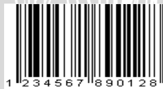
Gambar 2.14 Barcode tipe EAN
