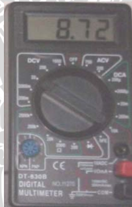
Gambar 5.3. Tegangan line telepon saat off hook
