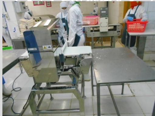
**Gambar 17.** *Metal detector machine*
