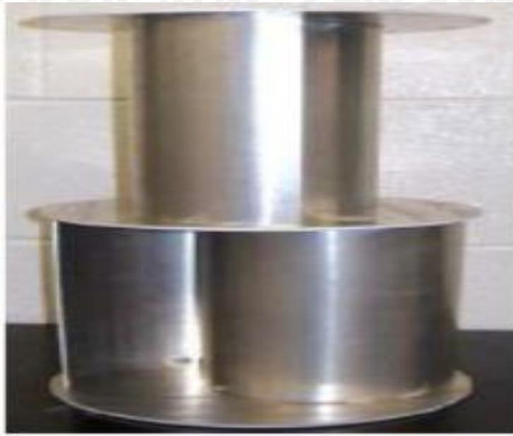
Gambar 5. Turbin Savonius (Alam dkk, 2009)
