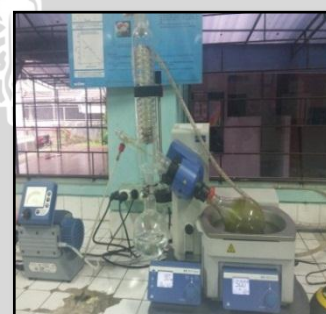
Rotary vacuum evaporator
