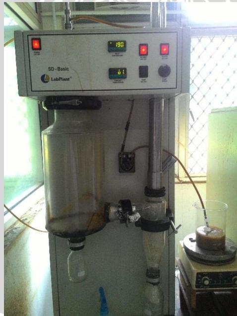
**Gambar 6.** Alat *Spray dryer*.
