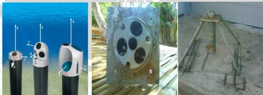
Gambar 6. ADCP Nortek Aquadop
