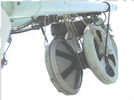
Gambar 8. *Hydraulic Power Block*
