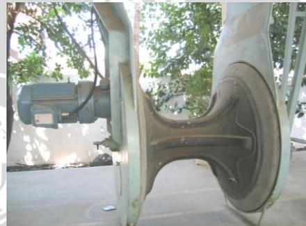
Gambar 9. *Electric Power Block*
