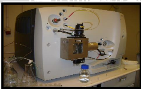
**Gambar 7. Liquid Chromatography Mass Spectrophotometry merk Waters tipe LCT Premier XE**
