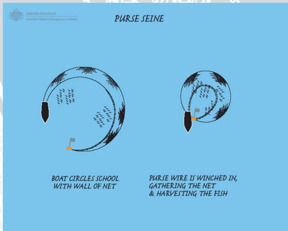
Gambar 2. Proses Pengoperasian alat tangkap purse seine ( www.afma.gov.au, 2007)
