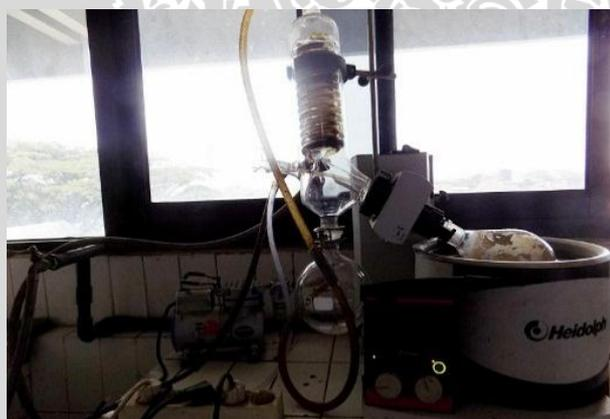
Gambar Lampiran 2. Rotary Vacum Ovaporator
