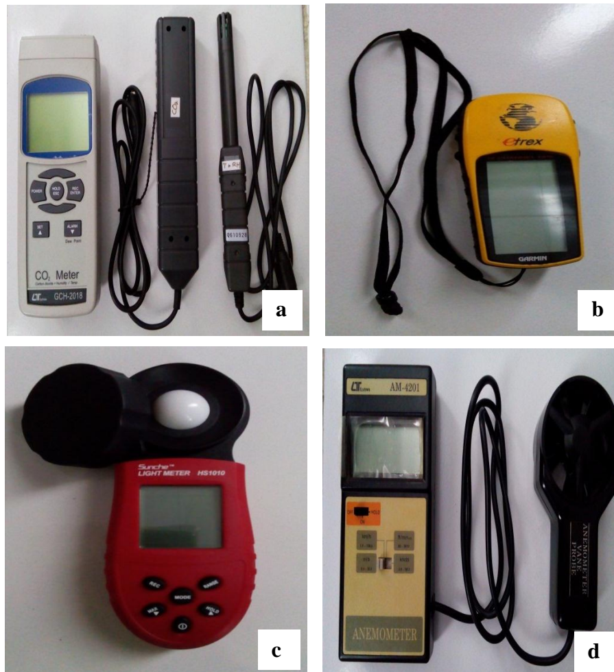
Gambar 5. Alat Pengukur Iklim (a) CO 2 Meter Lutron GC – 2018; (b) GPS Garmin; (c) Sunche Light Meter Tipe HS1010; (d) Anemometer Tipe AM-4201
