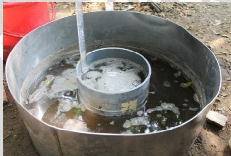
Gambar 1. Pengukuran Laju Infiltrasi (Double Ring Infiltrometer)
