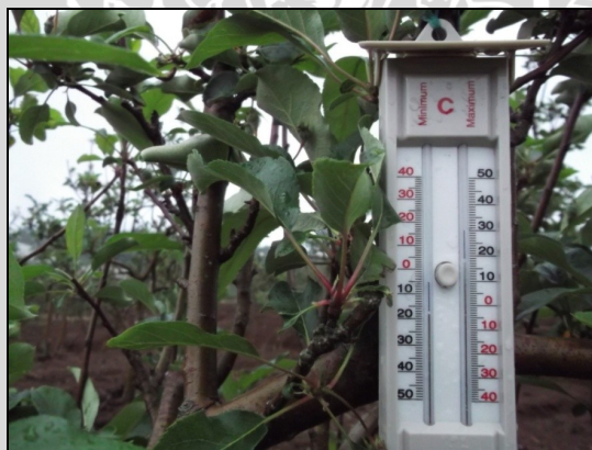
Gambar 18. Termometer Maximum-Minimum ( Six Bellani )
