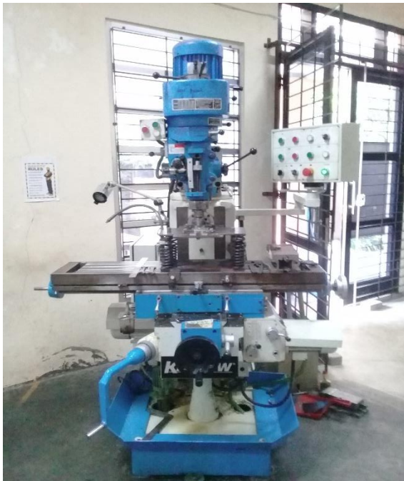
Gambar 3.1 Universal milling machine X6328B
