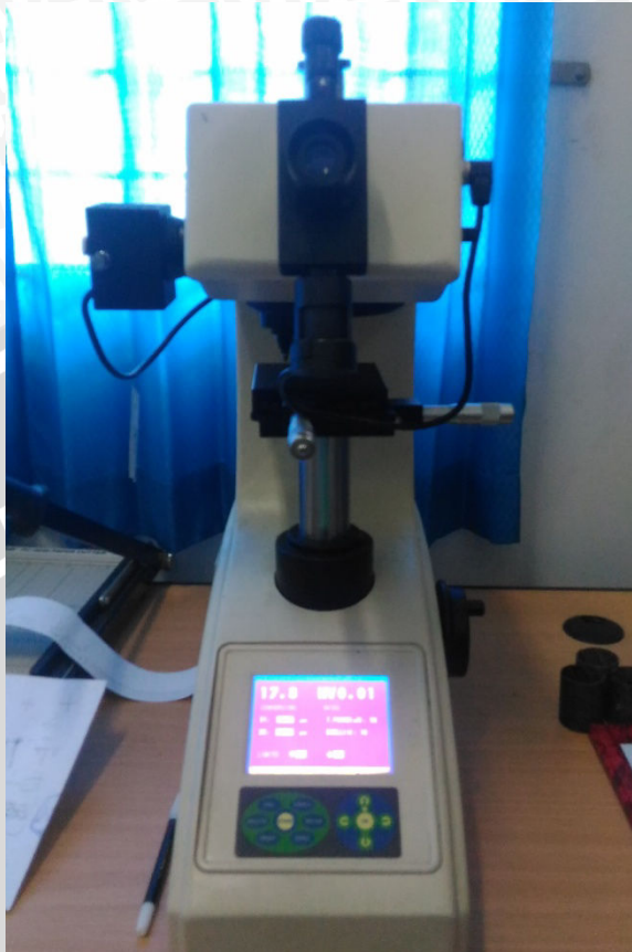
Gambar 4.2 Micro Hardness Tester merk Wilson Hardness Model: 402MVD
