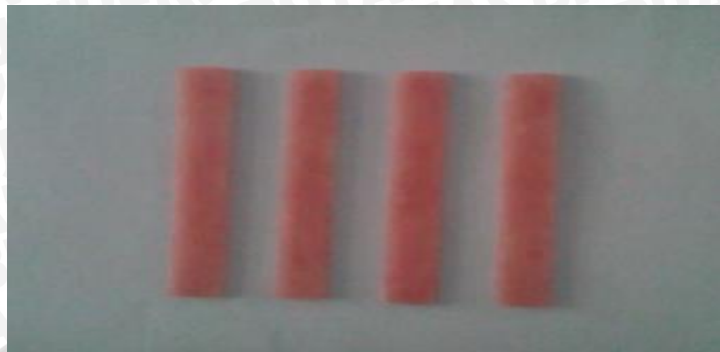
Gambar 4.1 Lempeng Heat Cured Acrylic Resin Ukuran 65 mm x 10 mm x 2,5 mm
