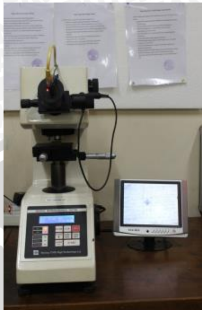
Gambar 4.2 Digital Micro Vickers Hardness Tester TH712
