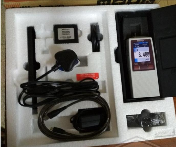
Gambar 3.2 Surface roughness tester
