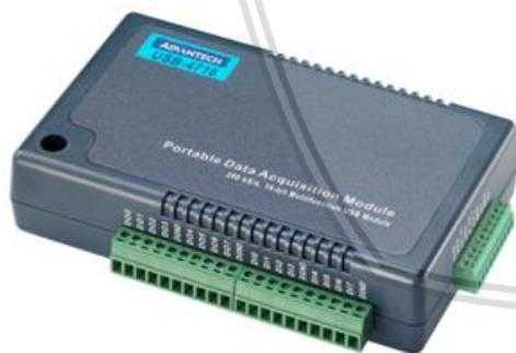
Gambar 3.2 Advantech USB-4718 data logger
