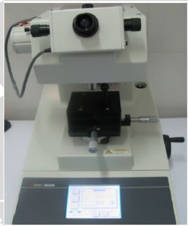
Gambar 2.9 Vickers Microhardness Device (Golpayegani, 2012)
