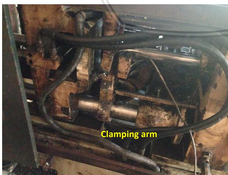
Gambar 7: penampang unit *driver ejection & clamping*
