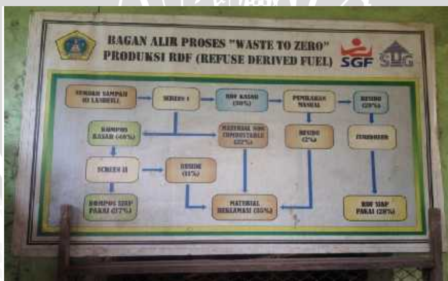
Gambar 12. Alur Proses “Waste to Zero” Produksi RDF ( Refuse Derived Fuel )
