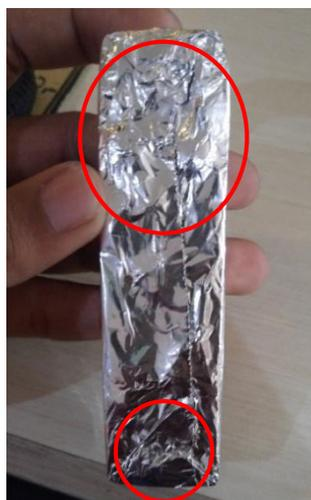
Gambar 7. Cacat Penutupan Aluminium Foil Tidak Rapi
