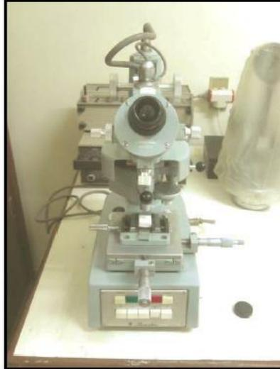
**Gambar 2.7** Micro Vickers Hardness Tester
