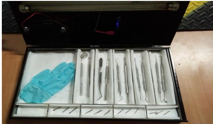
Gambar 2.6 Prototipe DENTMOX "Dental Magic Box with Ultraviolet Basis Sterilizing Innovation saat dibuka
