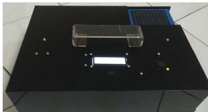
Gambar 2.5 Prototipe DENTMOX "Dental Magic Box with Ultraviolet Basis Sterilizing Innovation t tampak atas
