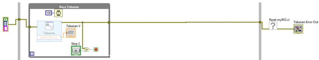
**Gambar 5.19** Potongan Program Baca Sensor Tekanan Air
