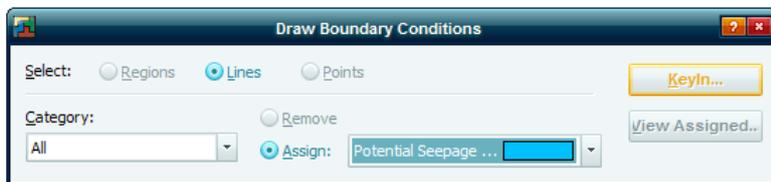
Gambar 2.48. Setting *Potential Seepage Face* pada *Keyin Boundary Conditions*
