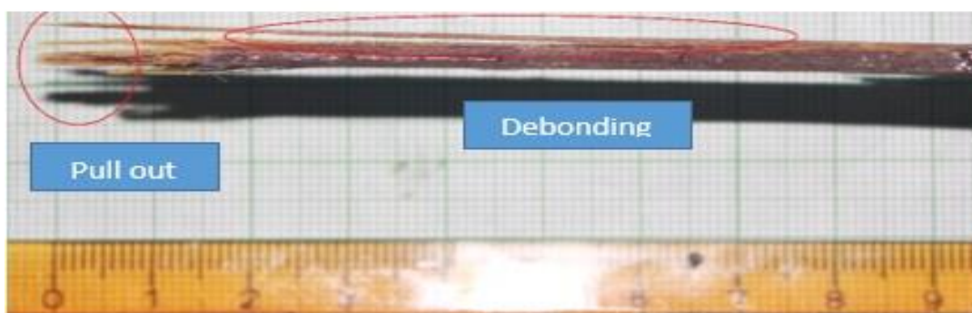
Gambar 4. 8 Foto permukaan patah spesimen matrik polyester single vacuum
