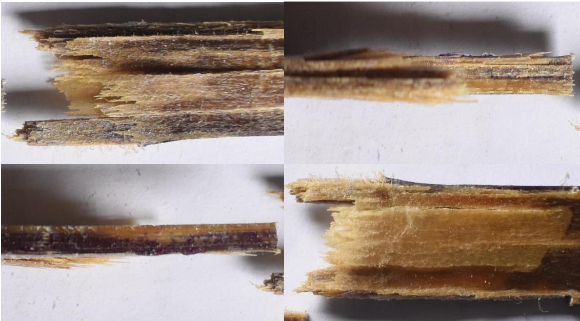
Gambar 4.7 Foto permukaan patah spesimen matrik polyester parallel vacuum
