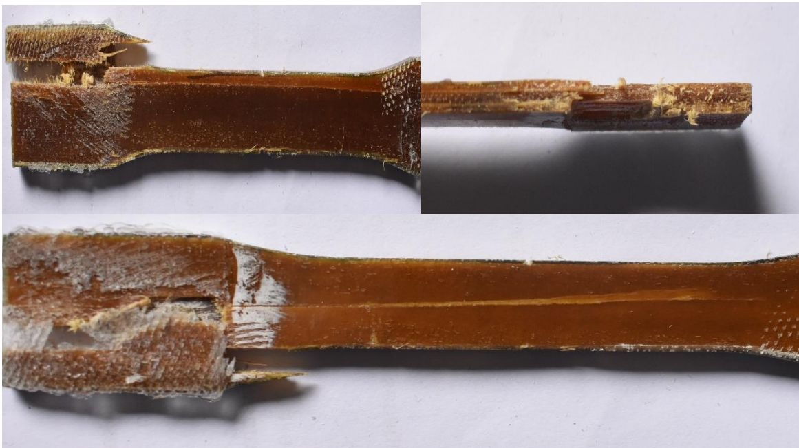
Gambar 4.4 Foto permukaan patah spesimen matrik epoxy parallel vacuum
