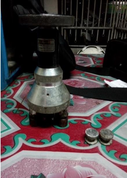
Gambar 3.6 Pull off test
