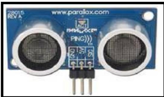
Gambar 2.16 Sensor Jarak Ultrasonik PING
