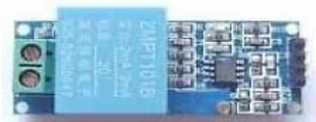
Gambar 1.14 Modul Sensor Tegangan ZMPT101B
