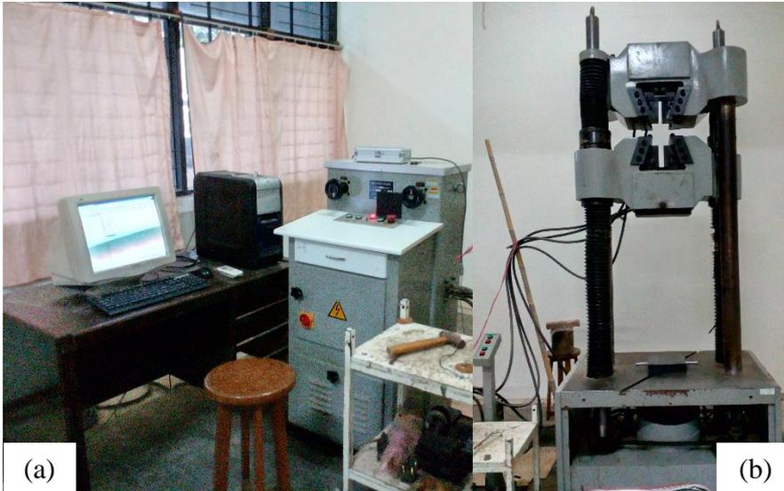
Gambar 3.4 Mesin Uji Tarik (a) *Display Controller* (b) *Specimen Holder*
