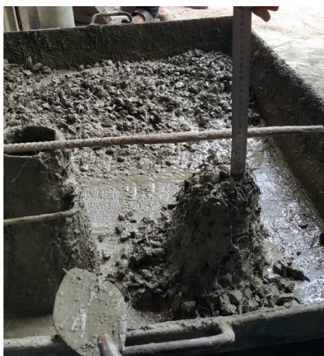
Gambar 4.1 Proses Uji Slump
