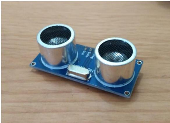
*Gambar 2.3* Sensor Ultrasonik HC-SR04
