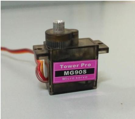
Gambar 2.11 Motor DC Servo
